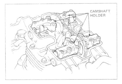
Install the camshaft holder bolts, but do not tighten them yet.
