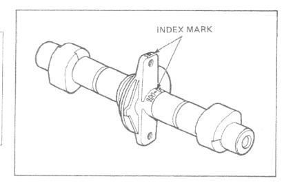
Lubricate the cylinder head cam bearing surfaces with molybdenum disulfide grease,
