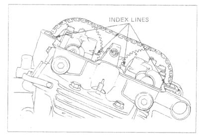
Slide the sprockets onto the camshaft flanges, and install the sprocket bolts in the exposed holes. Check that the sprocket index lines align at T1-3. Unlock the cam chain tensioner.
